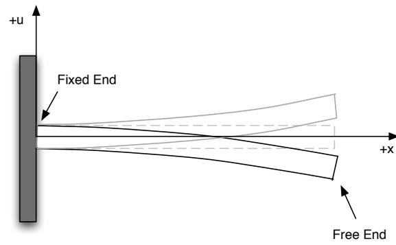
FIG. 1: The cantilever and coordinate system.
