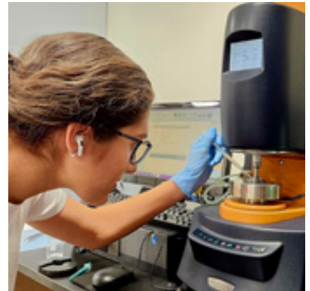
Aubrey Fessler measures and prepares a guar gum sample (a thickening agent commonly used in research) to test in a rheometer, a device that measures how materials flow and stretch.
